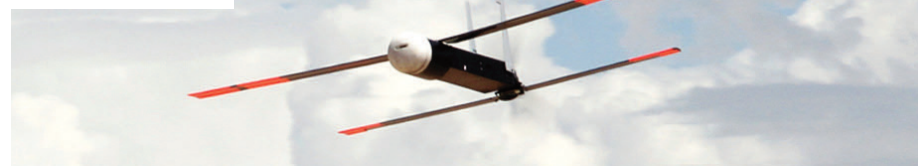
Initially, AFSOC will use Raytheon's Coyote small UAV on AC-130 gunships for the tactical off-board sensing mission.
